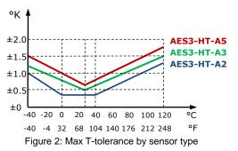
Note on accuracy: Allow 1 hour after power up for compensation swing in until described accuracy is reached.
