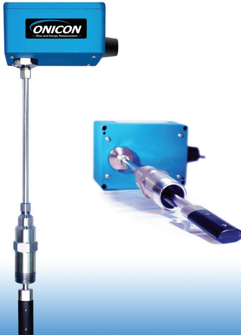
*ONICON's F-3500 series insertion electromagnetic flow meters are suitable for measuring electrically conductive liquids in a wide variety of applications. Each F-3500 provides a single analog output for flow rate, a high resolution frequency output to drive peripheral devices, a scalable pulse output for totalization, and an empty pipe alarm signal.*
